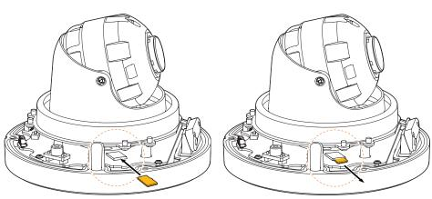
**NOTE:** Maximum SD Card size supported: Up to 1TB micro SD / FAT32. When inserting the SD card into the card slot, the SD card's contacts should be facing downward, as shown in the diagram.
